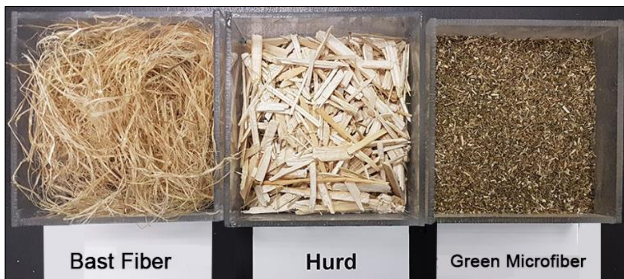
Figure 7 - Dry processing separation of bast fiber (left), hurd fiber (center), and green microfiber (right).
