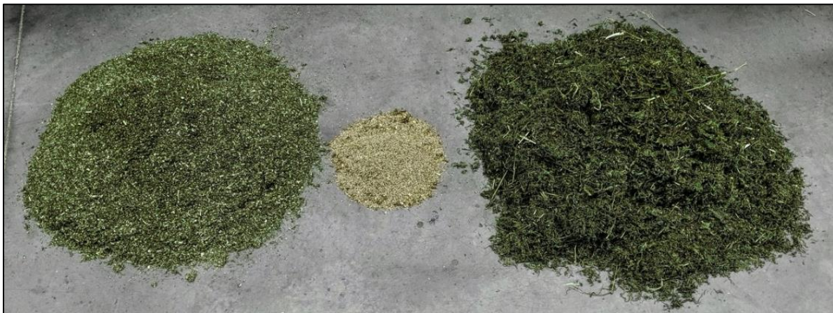
Figure 6 – Fresh/Green processing separation of High-CBD Fraction (left) from seeds (center) and Low-CBD Green Microfiber Fraction (right)
