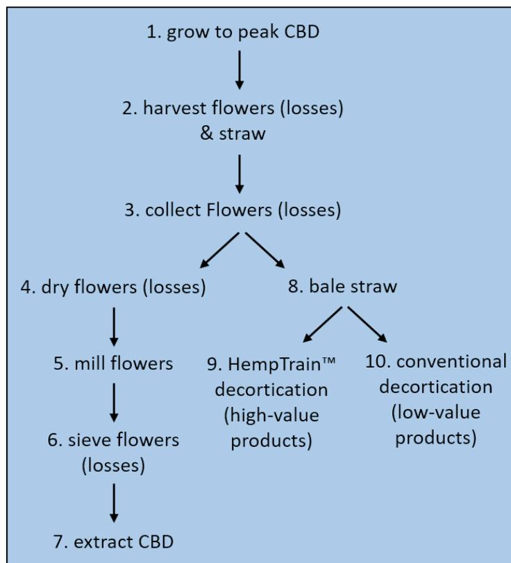
**Figure 7 - Double Header Harvesting Method Process Diagram**
