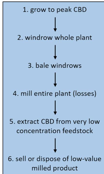
**Figure 8 - Whole Plant Milling Method Process Diagram**
