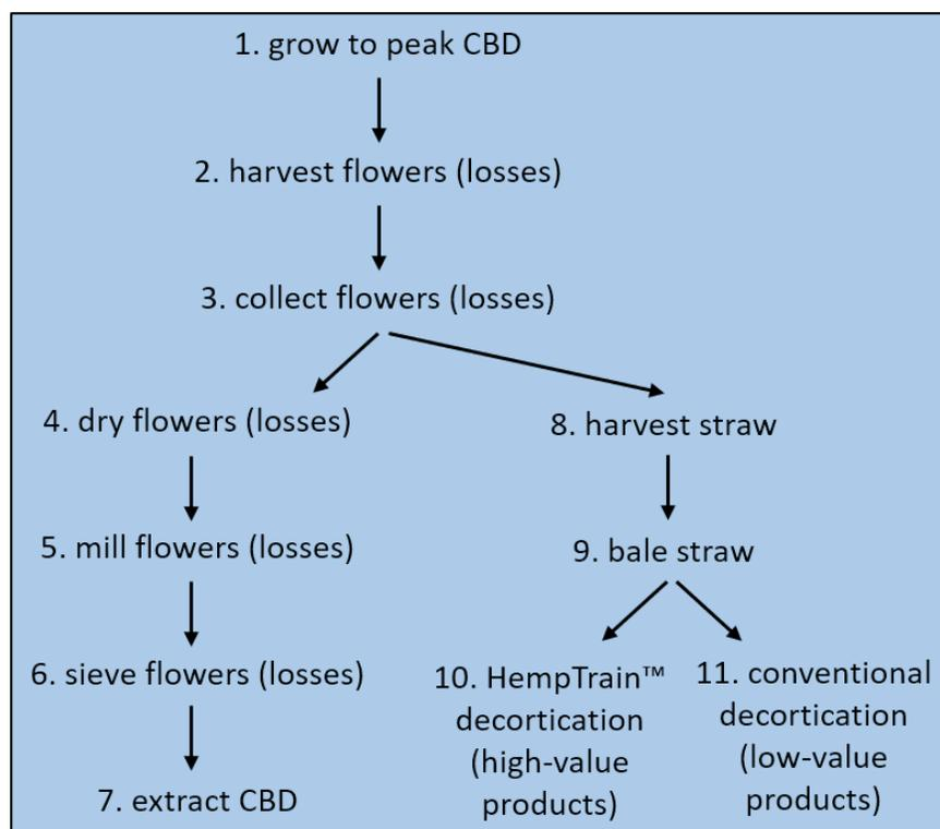
**Figure 4 - Two-Pass Harvesting Method Process Diagram**
