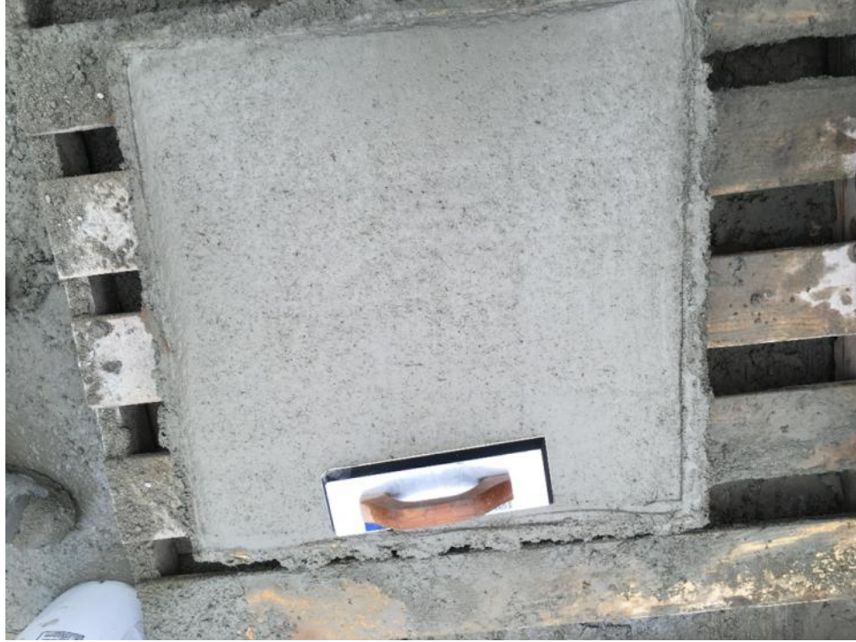
Figure E-17: NForce-Fiber wet-mix shotcrete finish: hard rubber float finish
