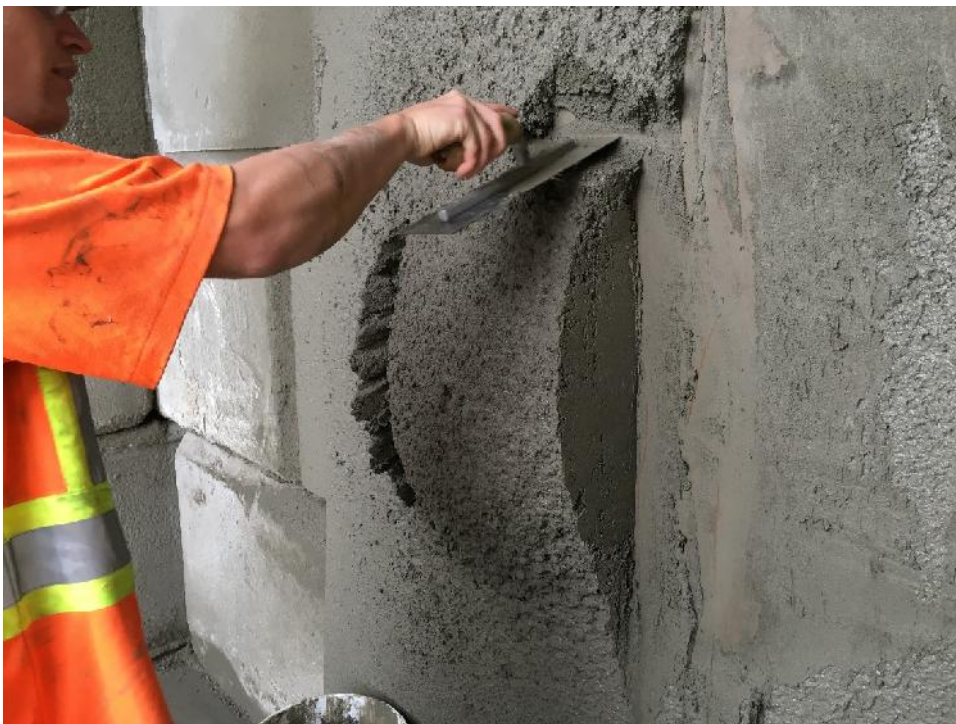
Figure B-10: Testing the cohesiveness and adhesion of the NForce-Fiber wet-mix shotcrete. Note that the shotcrete adhered to the wall and no sloughing occurred after multiple cuts with a steel trowel
