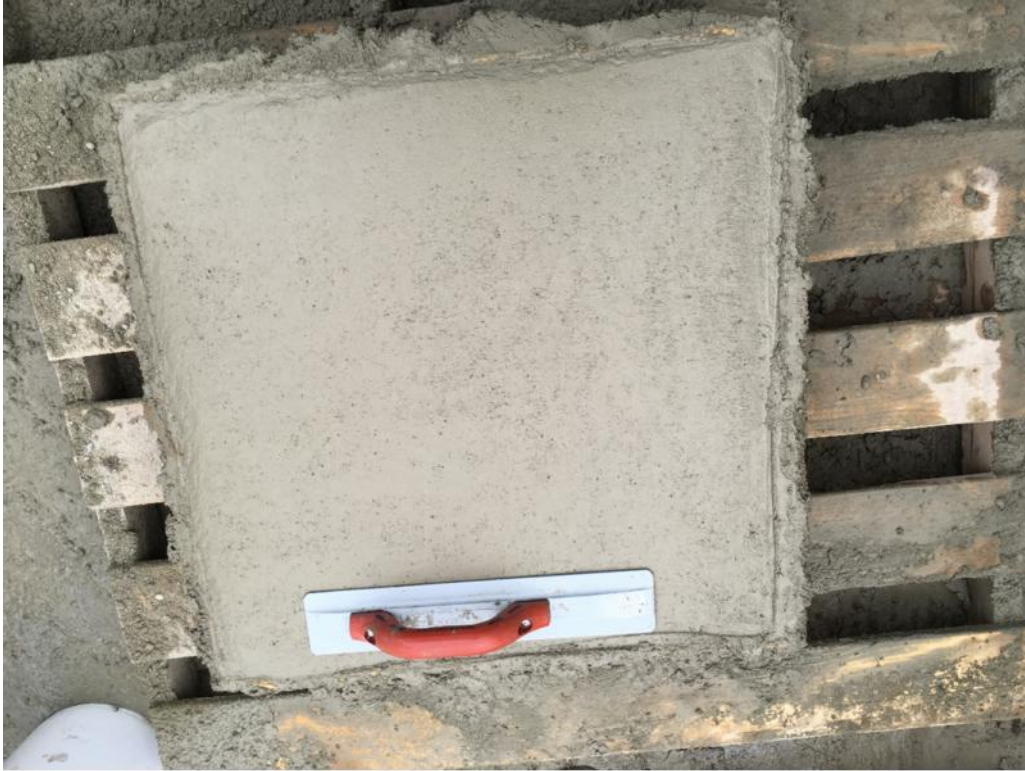
Figure E-15: NForce-Fiber wet-mix shotcrete finish: magnesium finish
