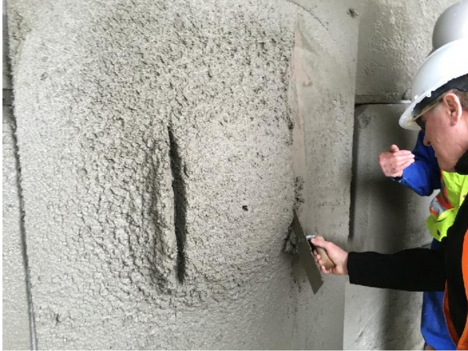
Figure B-9: Testing the cohesiveness of the NForce-Fiber wet-mix shotcrete
