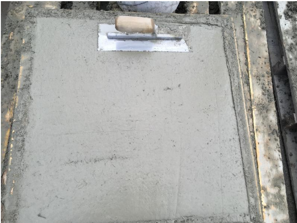
Figure E-8: Microsynthetic fiber wet-mix shotcrete finish: steel trowel finish
