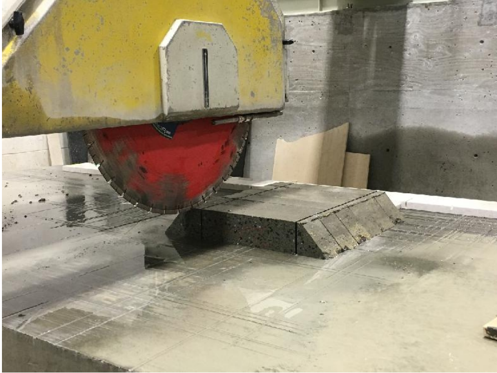
Figure B-15 Test panels were saw-cut to beams
