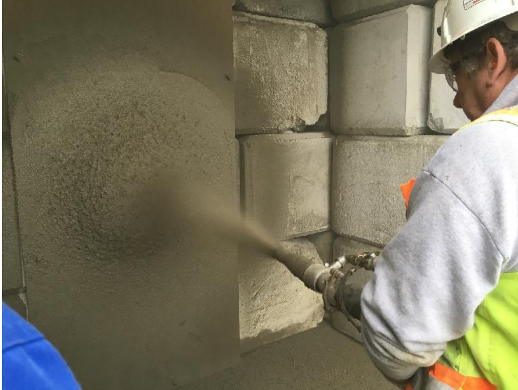
Figure B-5: Vertical rebound test for plain wet-mix shotcrete
