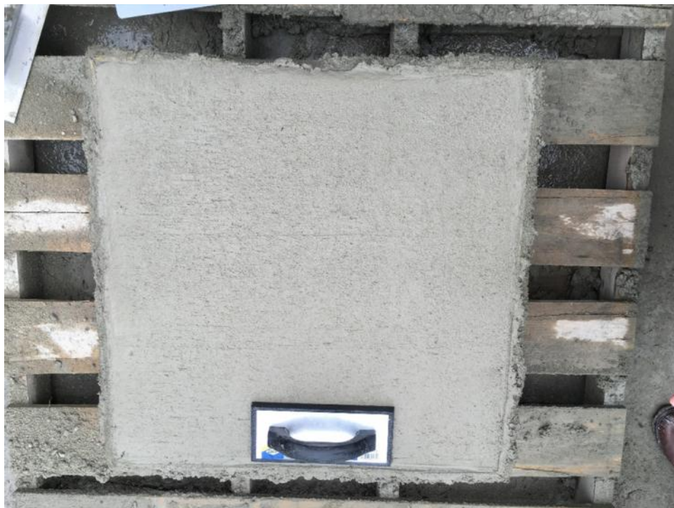
Figure E-18: NForce-Fiber wet-mix shotcrete finish: textured rubber float finish
