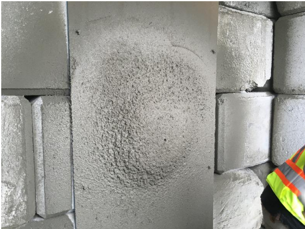
Figure B-6: Plain wet-mix shotcrete vertical thickness build-up
