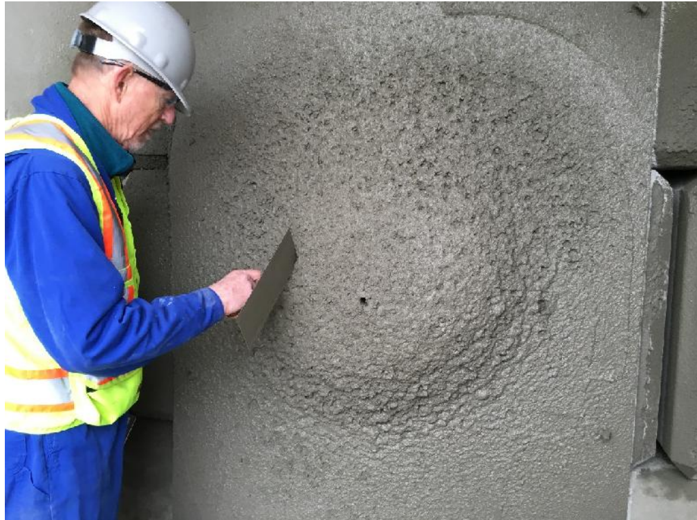
Figure B-8: Testing the cohesiveness of the NForce-Fiber wet-mix shotcrete
