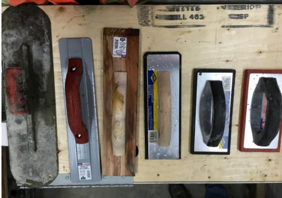
Figure E-1: Finishing tools (left to right): steel trowel, magnesium trowel, wood float, hard rubber float, textured rubber float, sponge float
