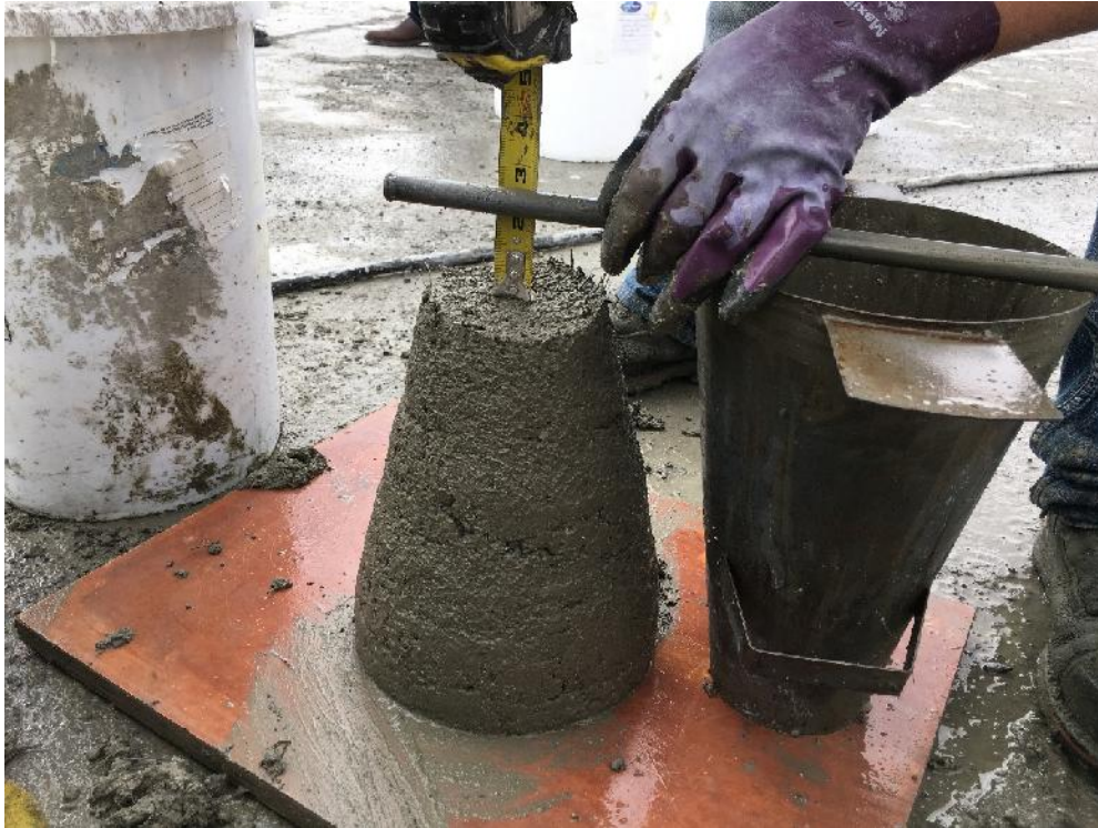
Figure B-11: Slump test for microsynthetic fiber wet-mix shotcrete
