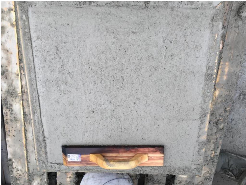
Figure E-10: Microsynthetic fiber wet-mix shotcrete finish: wood float finish
