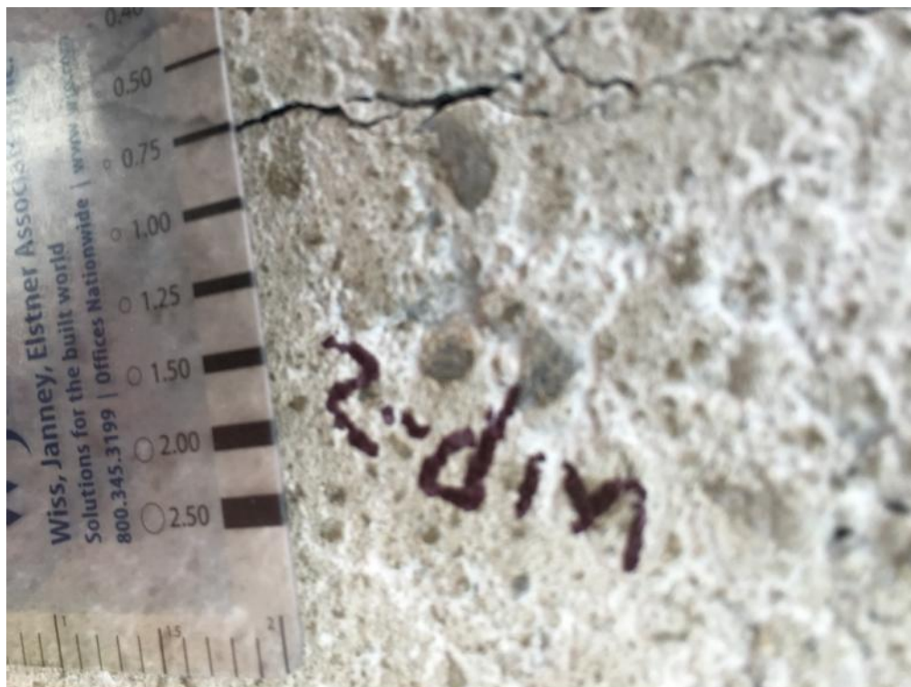
Figure D-2: Plain wet-mix shotcrete panel #2, 0 kg/m 3 fiber, crack width of 0.75 mm
