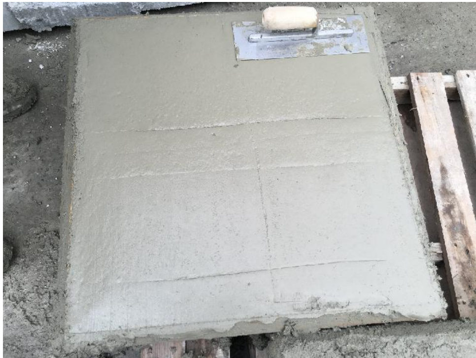
Figure E-2: Plain wet-mix shotcrete mix finish: steel trowel finish
