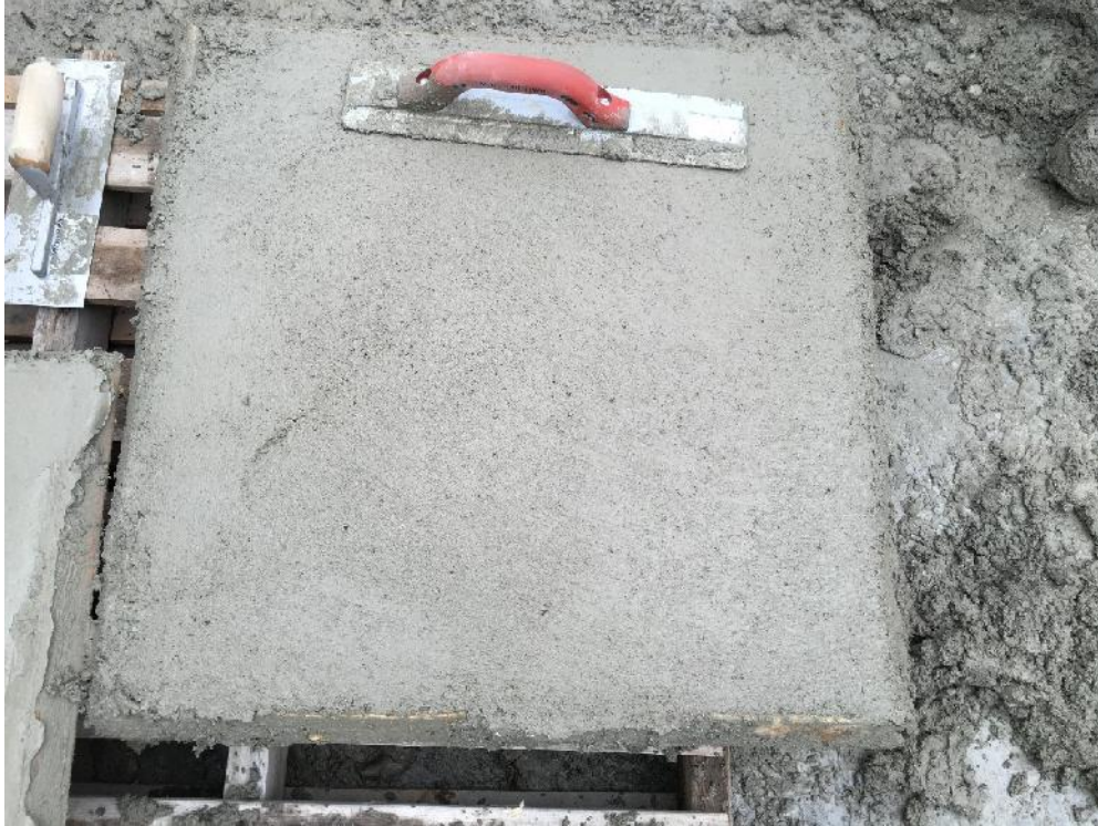
Figure E-3: Plain wet-mix shotcrete mix finish: magnesium finish
