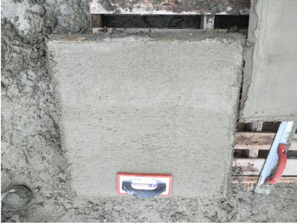
Figure E-7: Plain wet-mix shotcrete mix finish: sponge float finish
