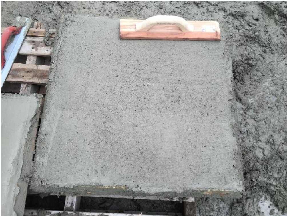
Figure E-4: Plain wet-mix shotcrete mix finish: wood float finish
