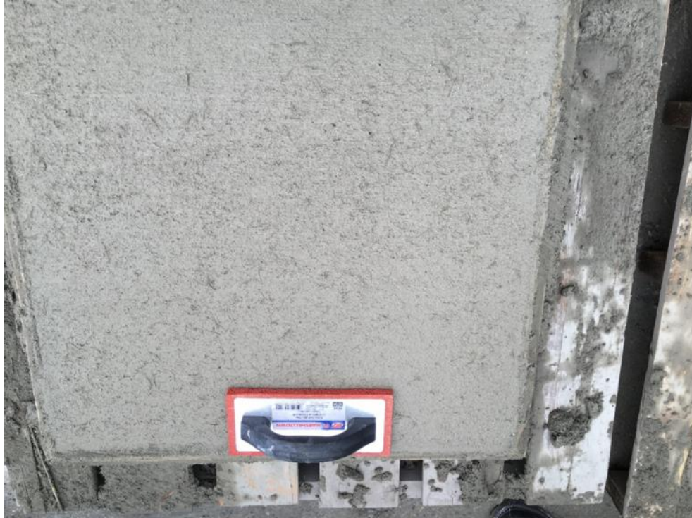
Figure E-13: Microsynthetic fiber mix finish: sponge float finish
