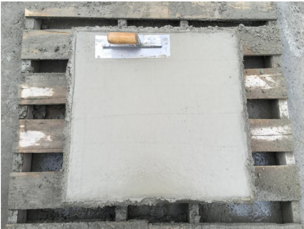
Figure E-14: NForce-Fiber wet-mix shotcrete finish: steel trowel finish
