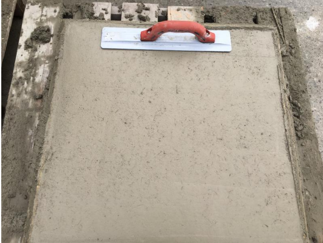
Figure E-9: Microsynthetic fiber wet-mix shotcrete finish: magnesium finish
