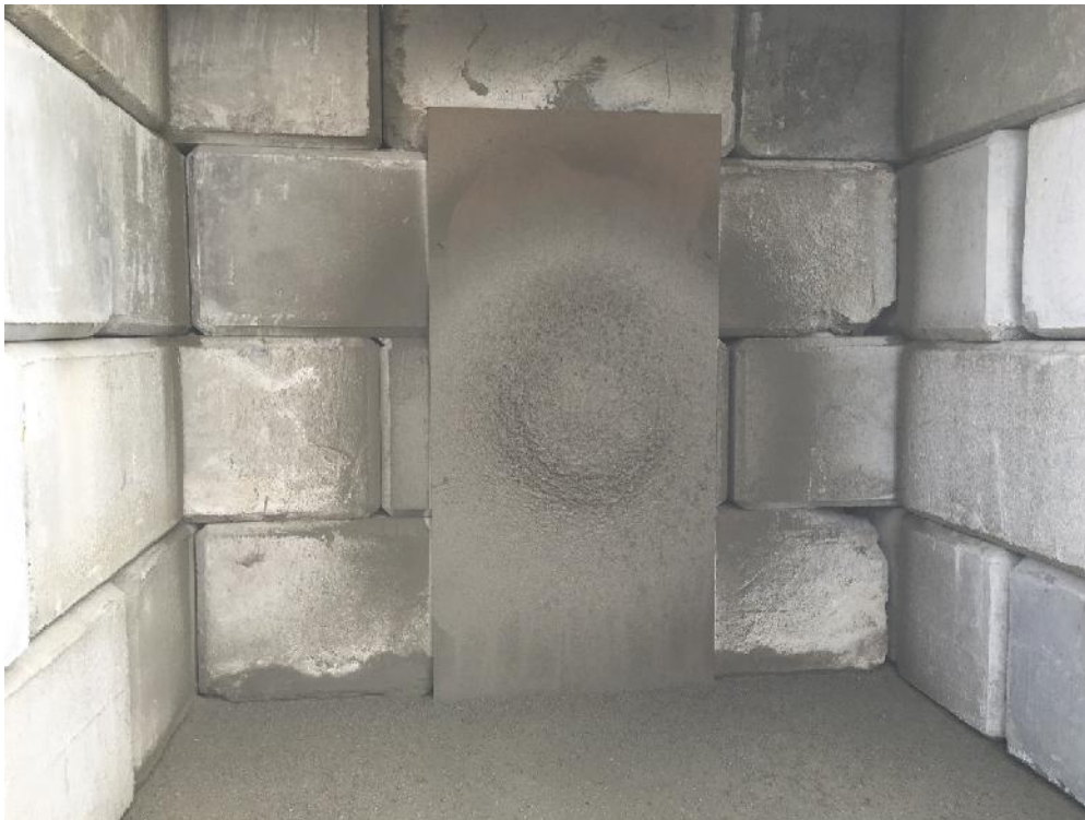
Figure B-12: Vertical rebound test and thickness build up for microsynthetic fiber wet-mix shotcrete
