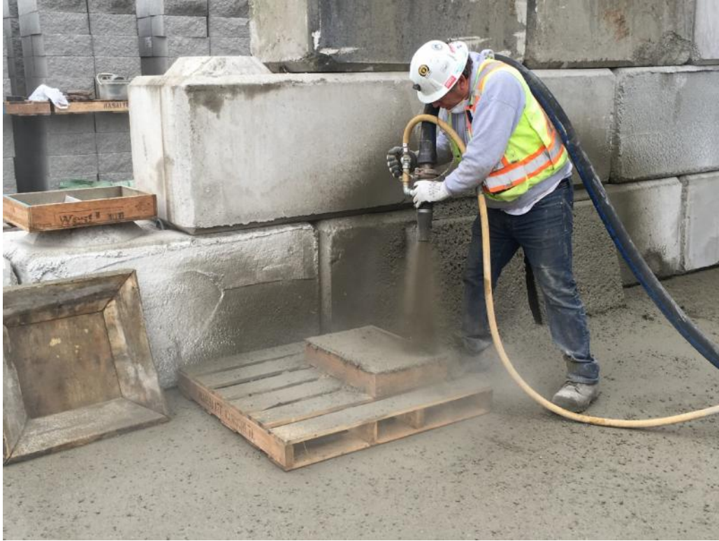
Figure B-3: Shooting panel for plastic shrinkage testing
