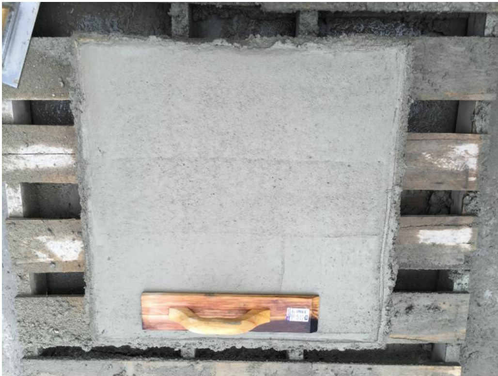
Figure E-16: NForce-Fiber wet-mix shotcrete finish: wood float finish
