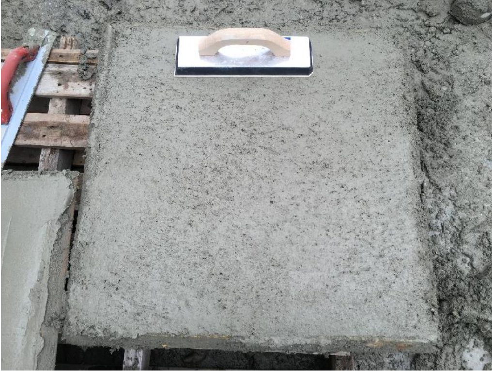
Figure E-5: Plain wet-mix shotcrete mix finish: hard rubber float finish
