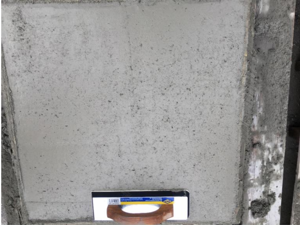
Figure E-11: Microsynthetic fiber wet-mix shotcrete finish: hard rubber float finish
