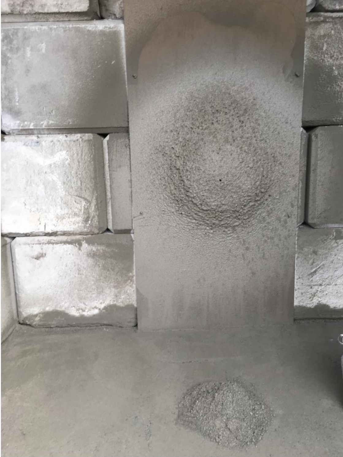
Figure B-14: Vertical rebound test: note the rebound materials on the floor were collected and weighed and materials adhered to the vertical wall were also collected and weighed.
