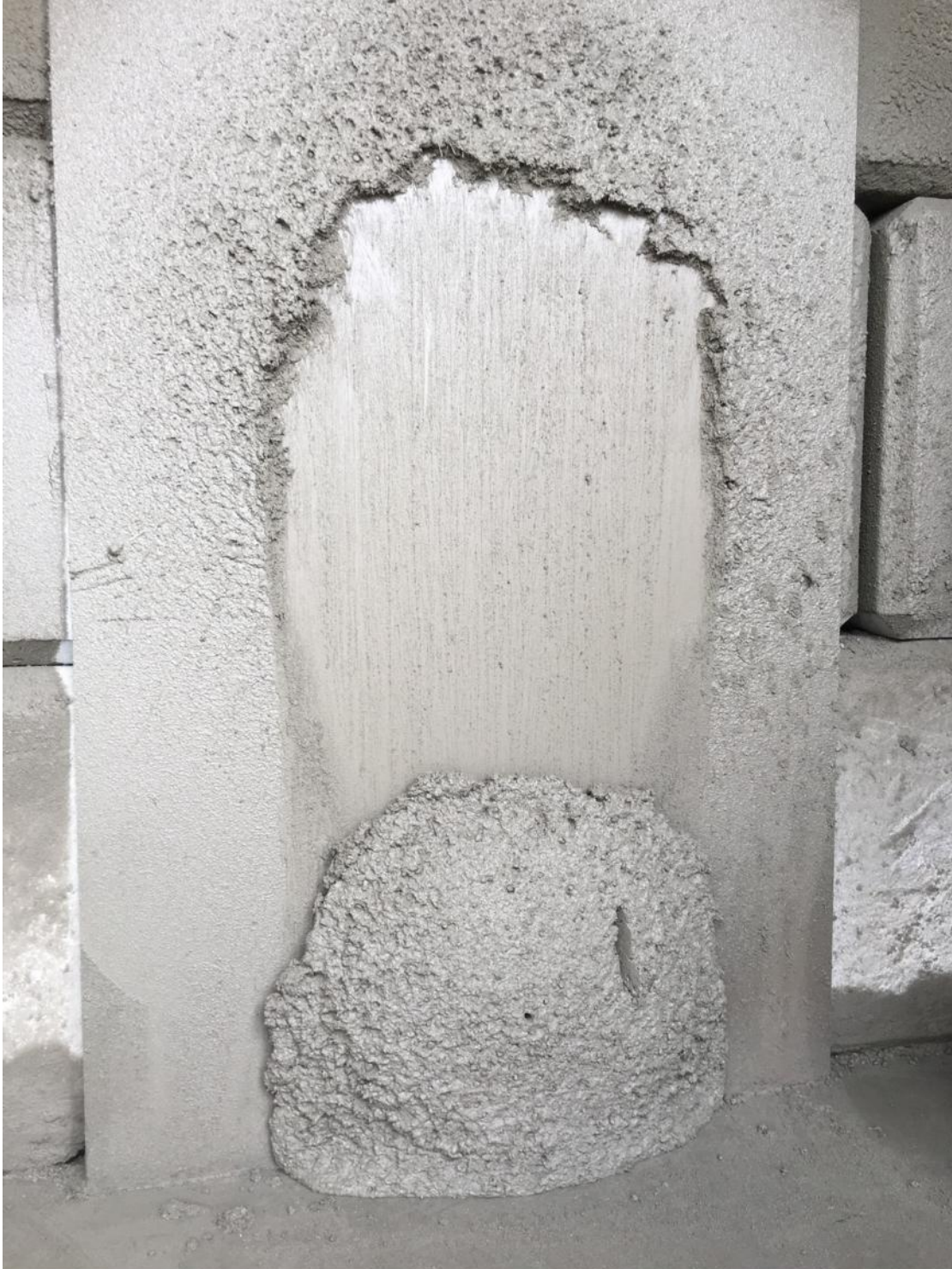
Figure B-13: Vertical thickness build up for microsynthetic fiber wet-mix shotcrete. Note that shotcrete sloughed after cut by a steel trowl
