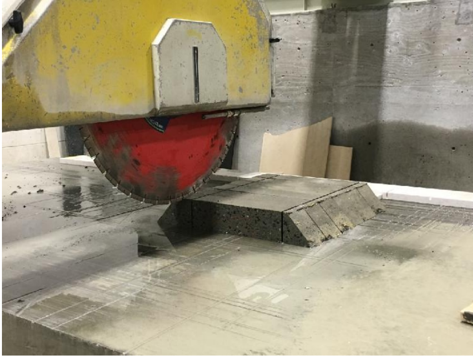
Figure B-22: Test panels saw-cut to produce beams
