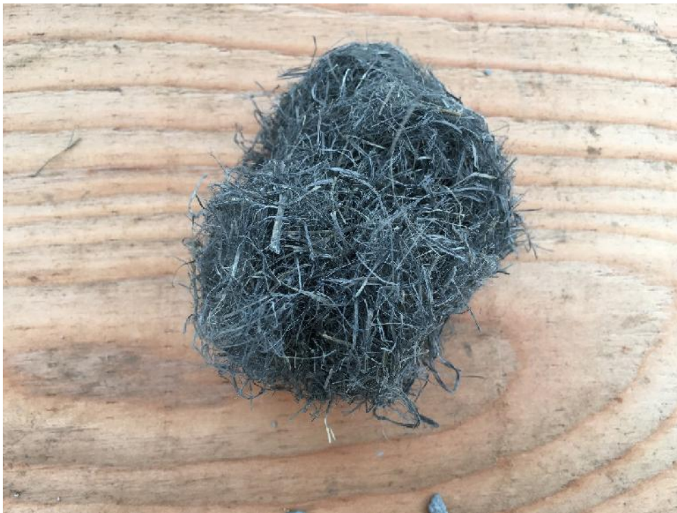
Figure B-13: NForced-Fiber retained on the hopper grid, a total weight of 8.5 gram, which is 0.56% by mass of the total batched fiber
