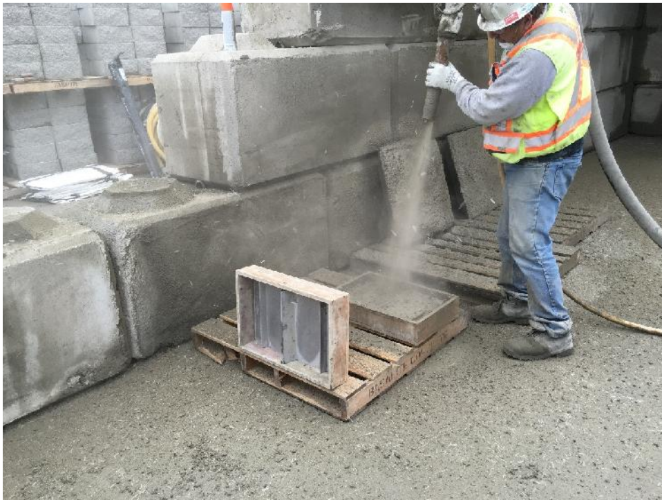
Figure B-5: Shooting panel for plastic shrinkage test
