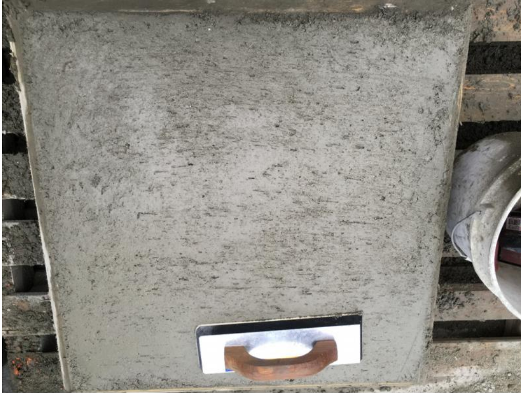
Figure E-17: NForce-Fiber dry-mix shotcrete finish: hard rubber float finish
