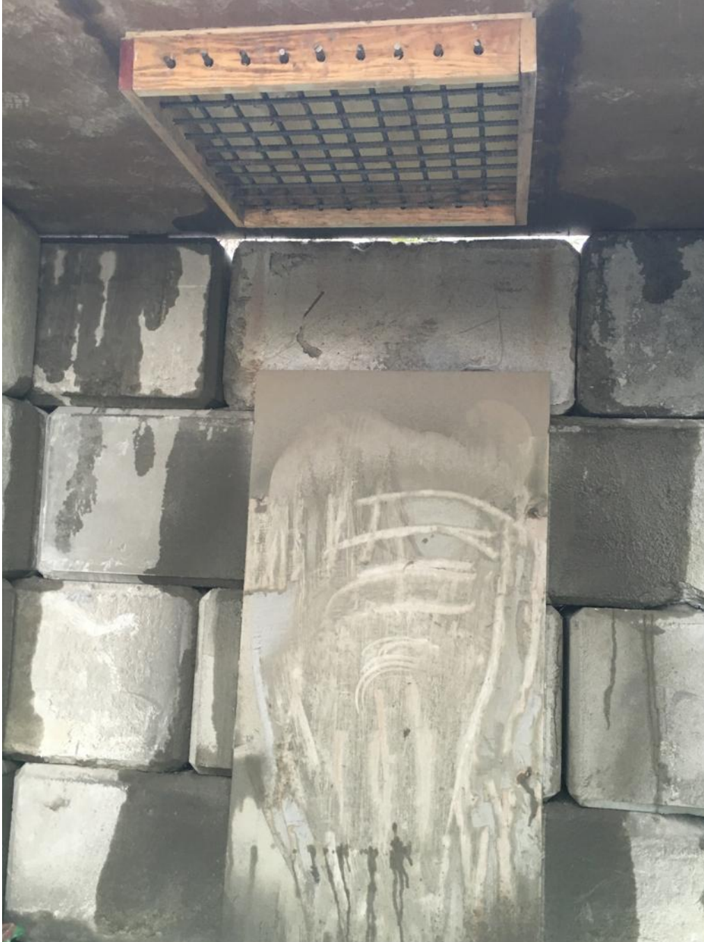
Figure B-3: Dry-Mix shotcrete rebound test set-up
