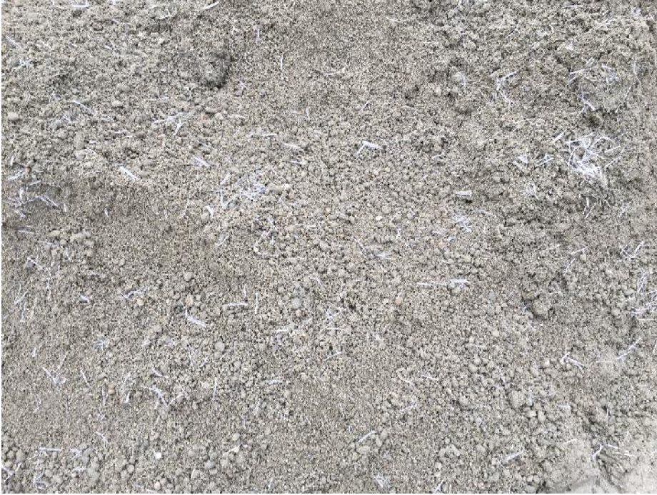
Figure B-16: Close look at the rebound for microsynthetic fiber reinforced dry-mix shotcrete
