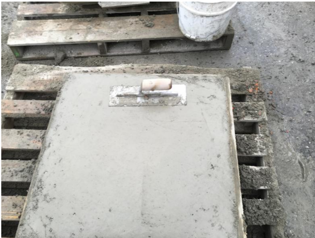
Figure E-14: NForce-Fiber dry-mix shotcrete finish: steel trowel finish
