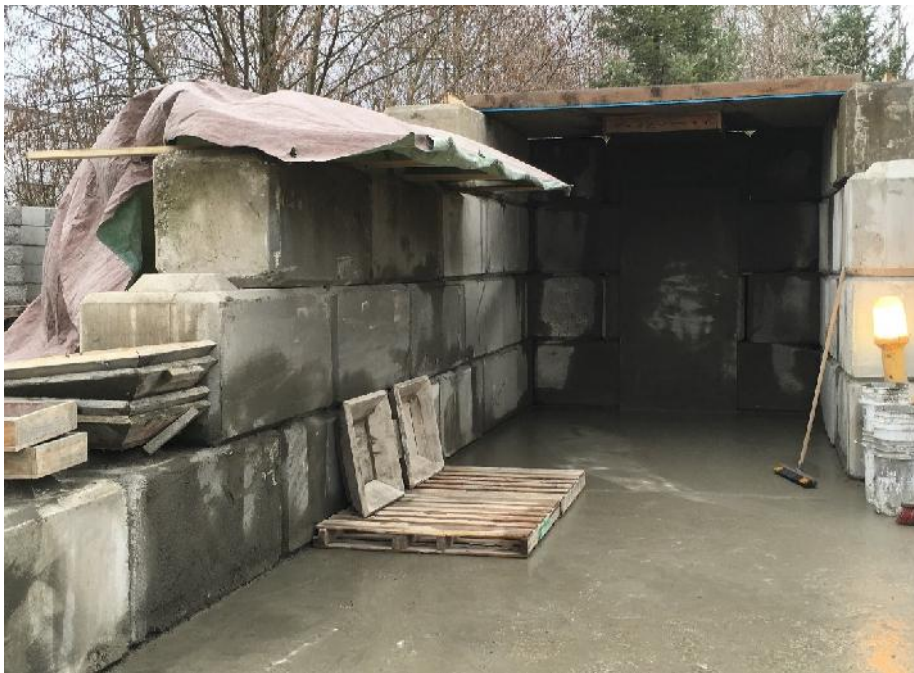
Figure. B-2: Setup for dry-mix shooting, including vertical and overhead rebound chamber, and test panels.
