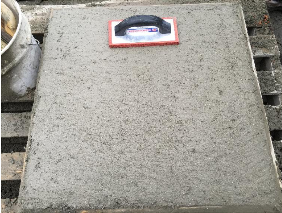
Figure E-19: NForce-Fiber dry-mix shotcrete finish: sponge float finish
