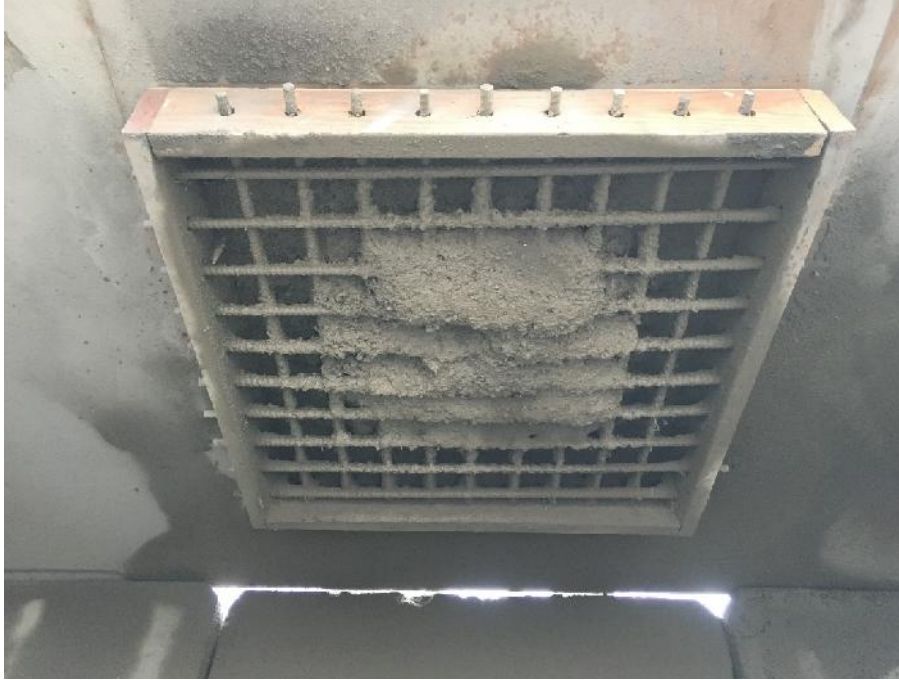
Figure B-18: Overhead shotcrete build-up for rebound test
