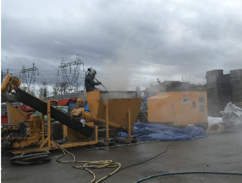
Figure B-20: Cleaning hopper after each mixture shot to avoid cross-contamination of mixes.
