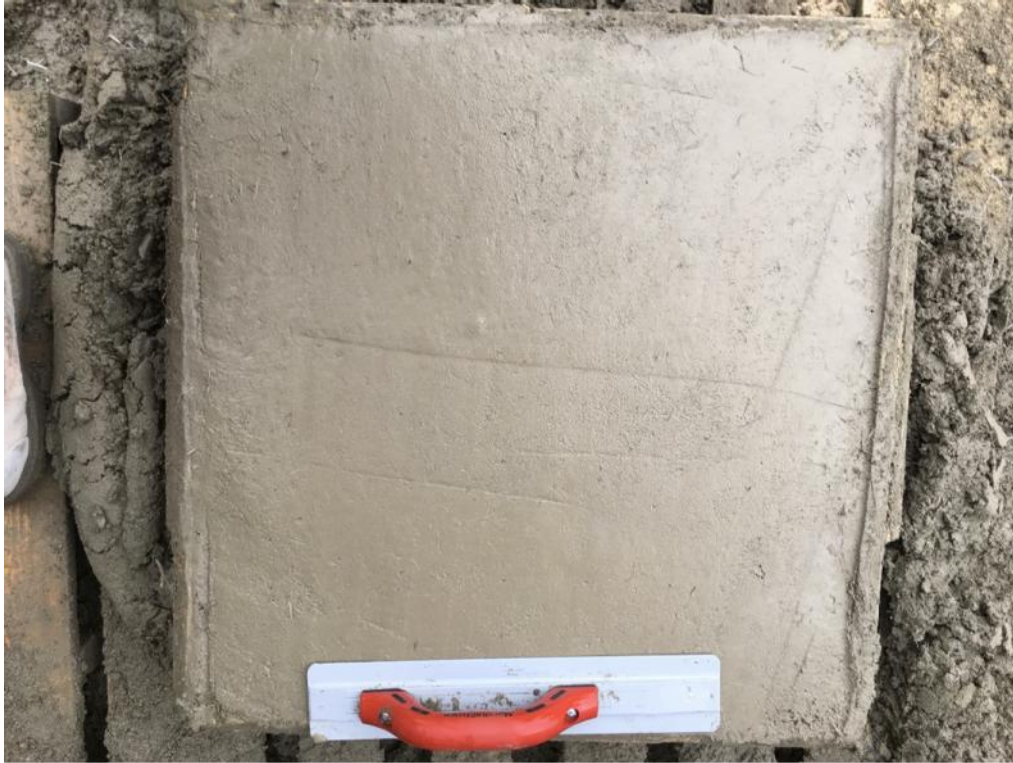
Figure E-9: Microsynthetic fiber dry-mix shotcrete finish: magnesium finish
