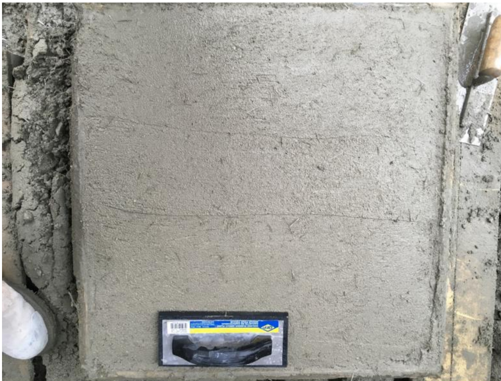
Figure E-12: Microsynthetic fiber dry-mix shotcrete finish: textured rubber float finish
