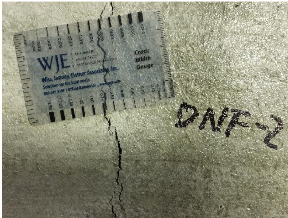
Figure D-4: NForce-Fiber panel #2, 2 kg/m 3 fiber, 0.75 mm crack width
