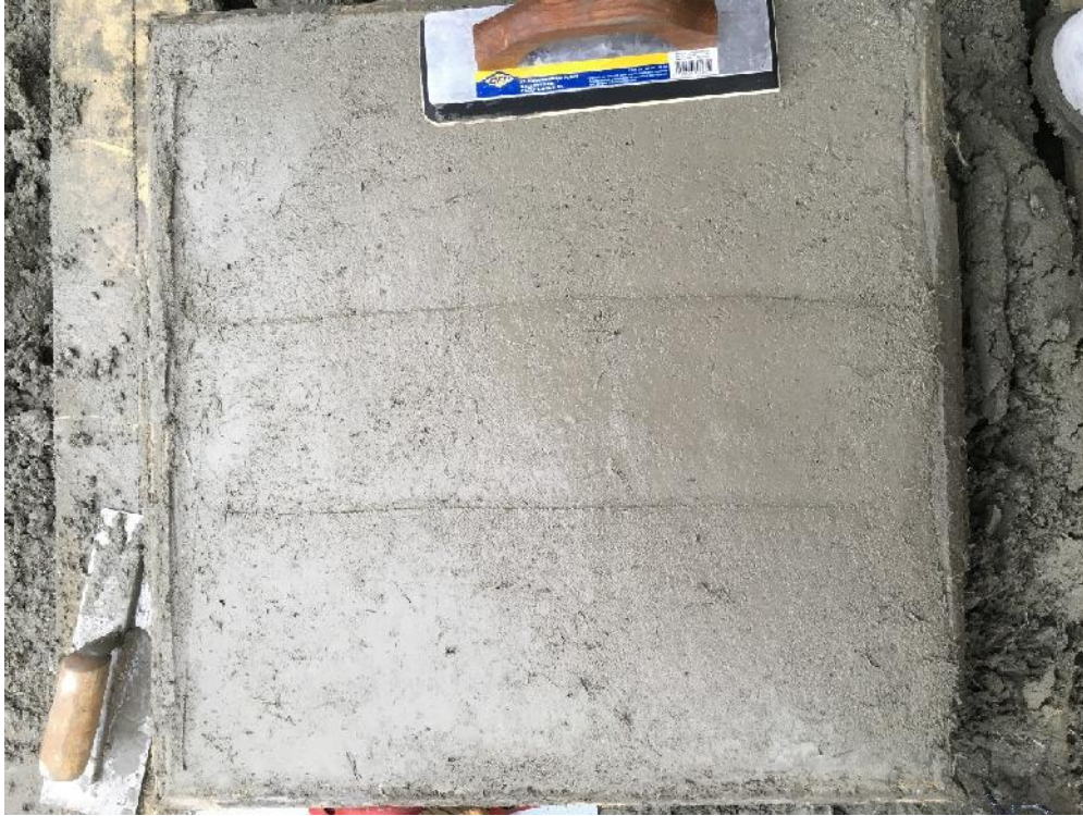
Figure E-11: Microsynthetic fiber dry-mix shotcrete finish: hard rubber float finish
