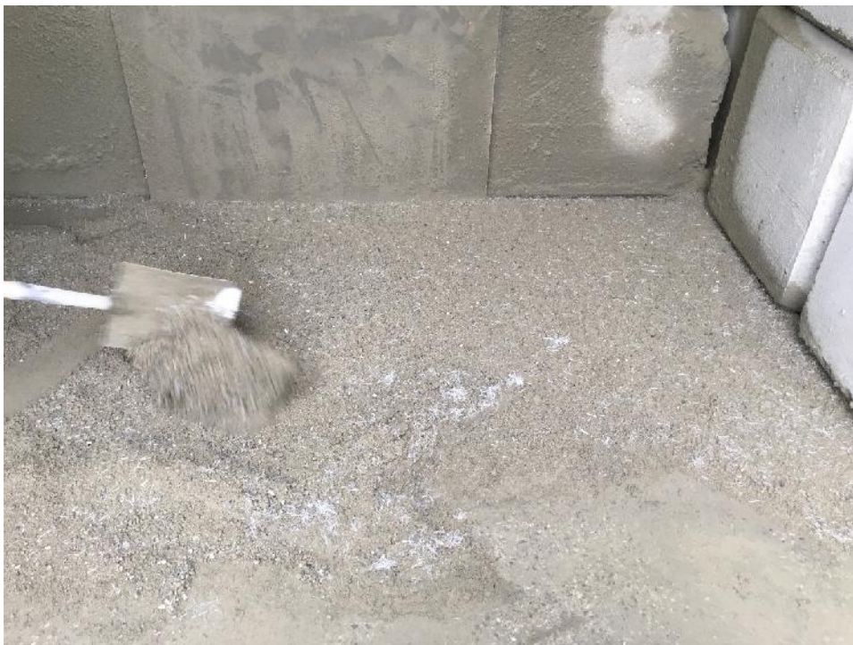
Figure B-15: Rebound test for microsynthetic fiber reinforced dry-mix shotcrete. Note that a significant amount of microsythetic fibers were blown out during shooting and not incorporated into the dry-mix shotcrete.
