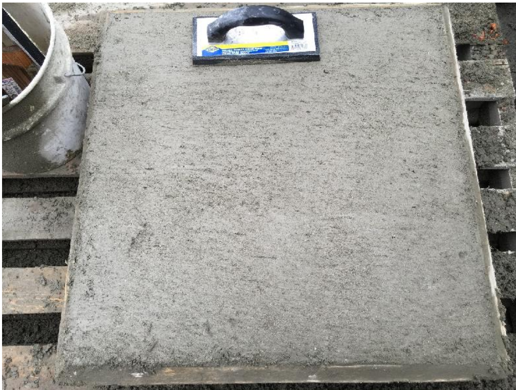
Figure E-18: NForce-Fiber dry-mix shotcrete finish: textured rubber float finish
