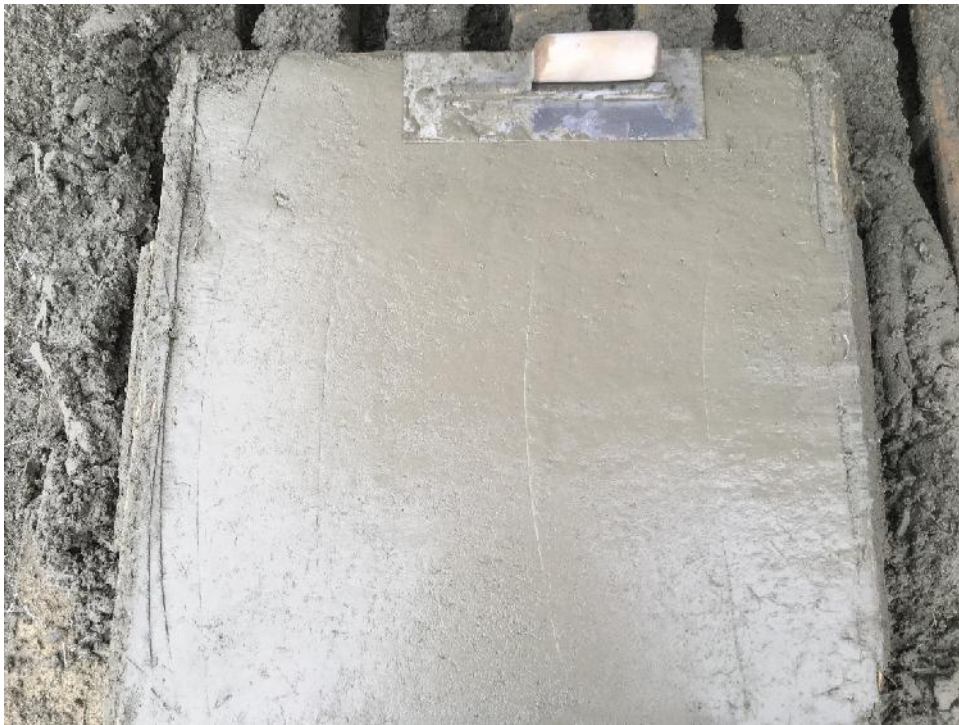
Figure E-8: Microsynthetic fiber dry-mix shotcrete finish: steel trowel finish
