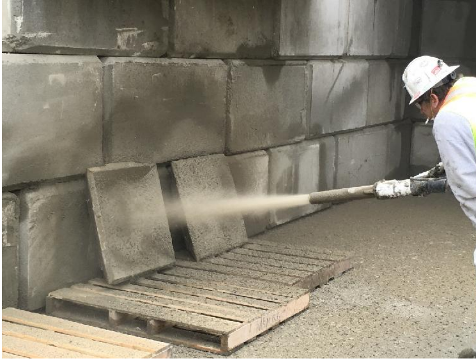
Figure B-14: Shooting microsythetic fibre reinforced dry-mix shotcrete, note that the fibers were blown out, deposited on the floor and not incorporated into the panel
