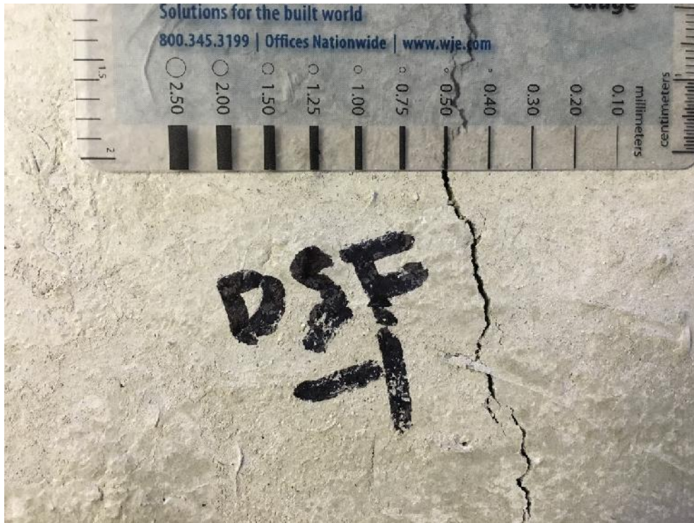
Figure D-5: Microsynthetic fiber panel #1, 1.35 kg/m 3 fiber, crack width of 0.50 mm
