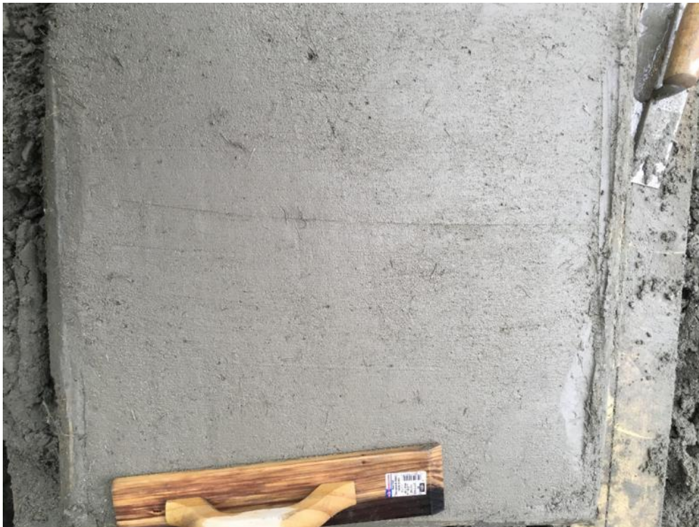
Figure E-10: Microsynthetic fiber dry-mix shotcrete finish: wood float finish
