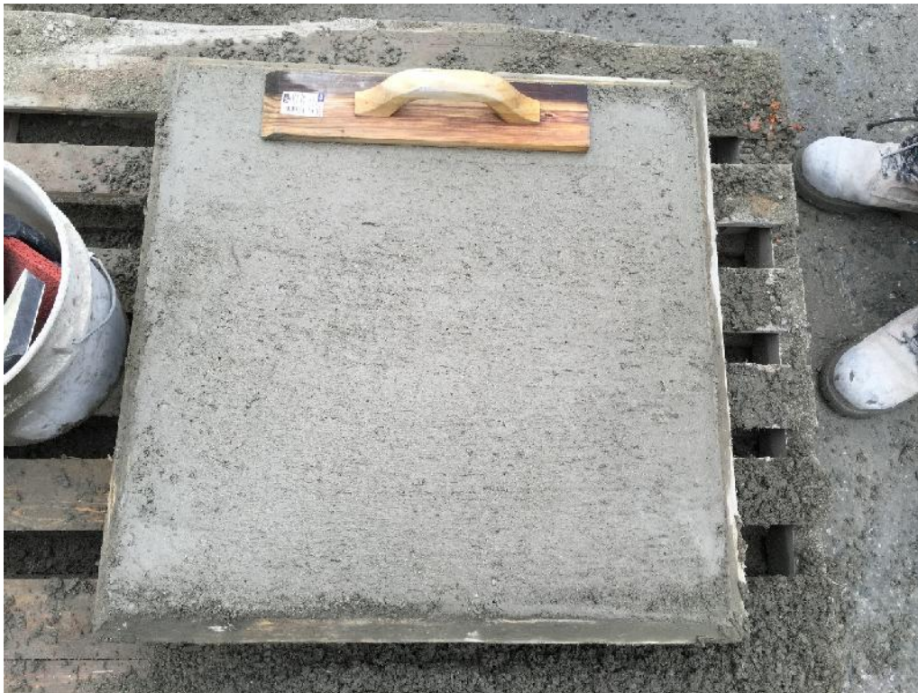
Figure E-16: NForce-Fiber dry-mix shotcrete finish: wood float finish
