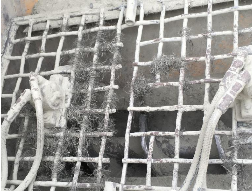
Figure B-12: NForce-Fiber retained on the grid of the hopper during shooting.
