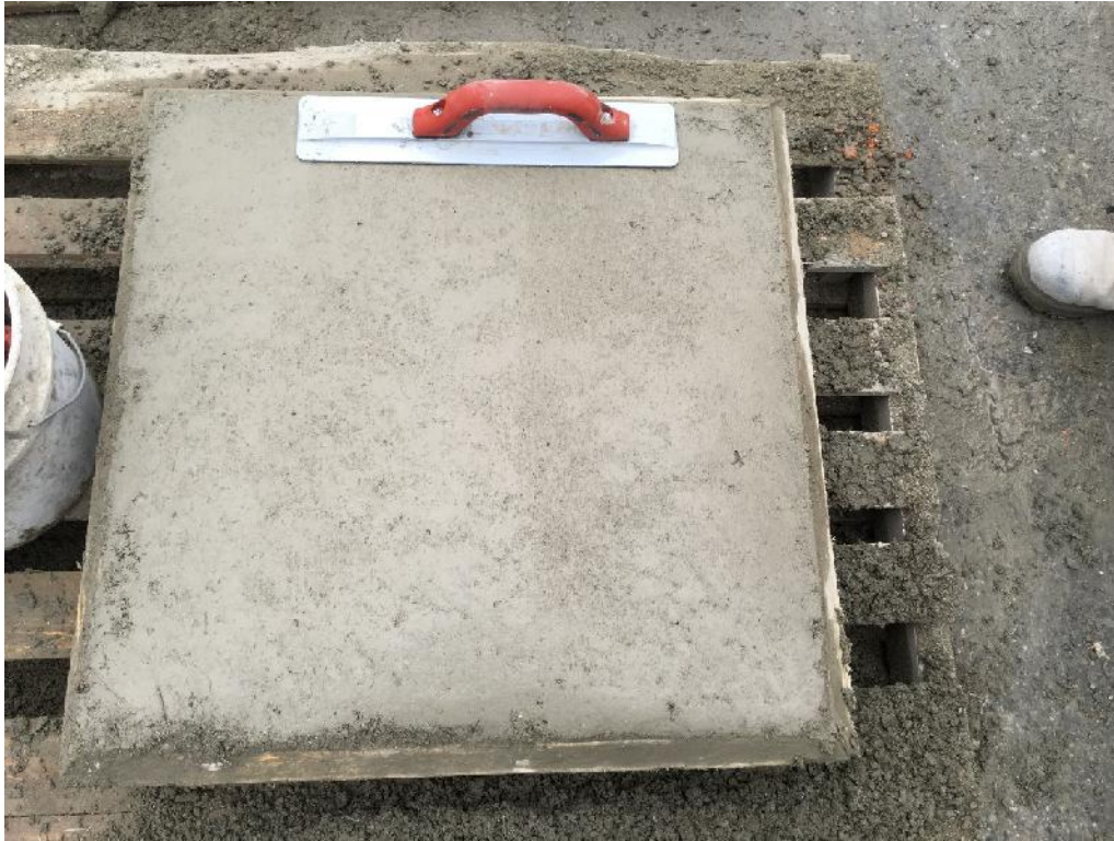
Figure E-15: NForce-Fiber dry-mix shotcrete finish: magnesium finish
