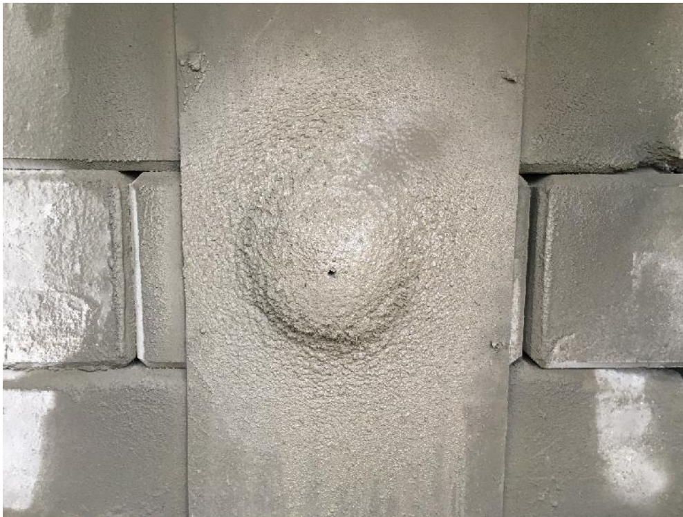
Figure B-7: Vertical build up with NForce-Fiber (2.0 kg/m 3 ) reinforced dry-mix shotcrete
