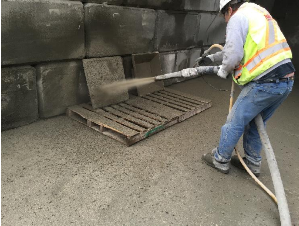
Figure B-4: Shooting test panels
