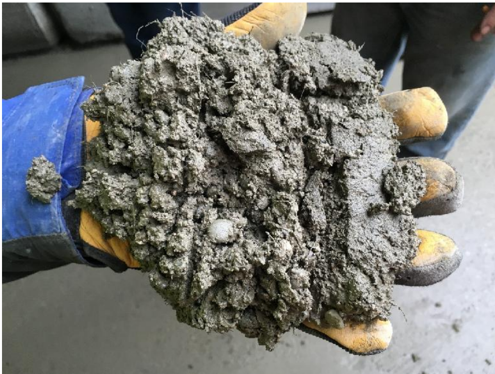
Figure B-11: NForce-Fiber reinforced dry-mix shotcrete after shoot
