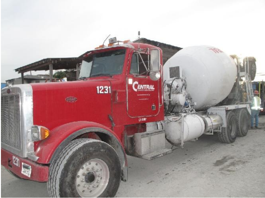
Fig.1 Ready-mix concrete truck used for mixing and supply of fiber-reinforced shotcrete
